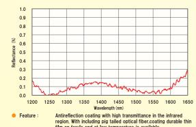
region. With including pig tailed optical fiber, coating durable thin film on ferule end at low temperature is available.
