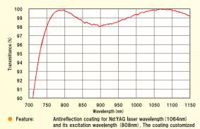
to your desired wavelength is possible Optical system for YAG laser etc.
